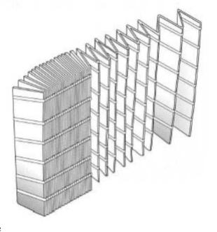
gas flow it bounces about due to collisions with molecules and again happens to slide close to a fiber and gets caught.
